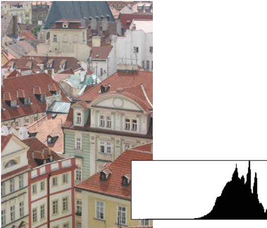
FIGURE 8.19 In a low-contrast image, the tones will be in the center of the histogram. Notice the lack of dark black or light gray tones.
